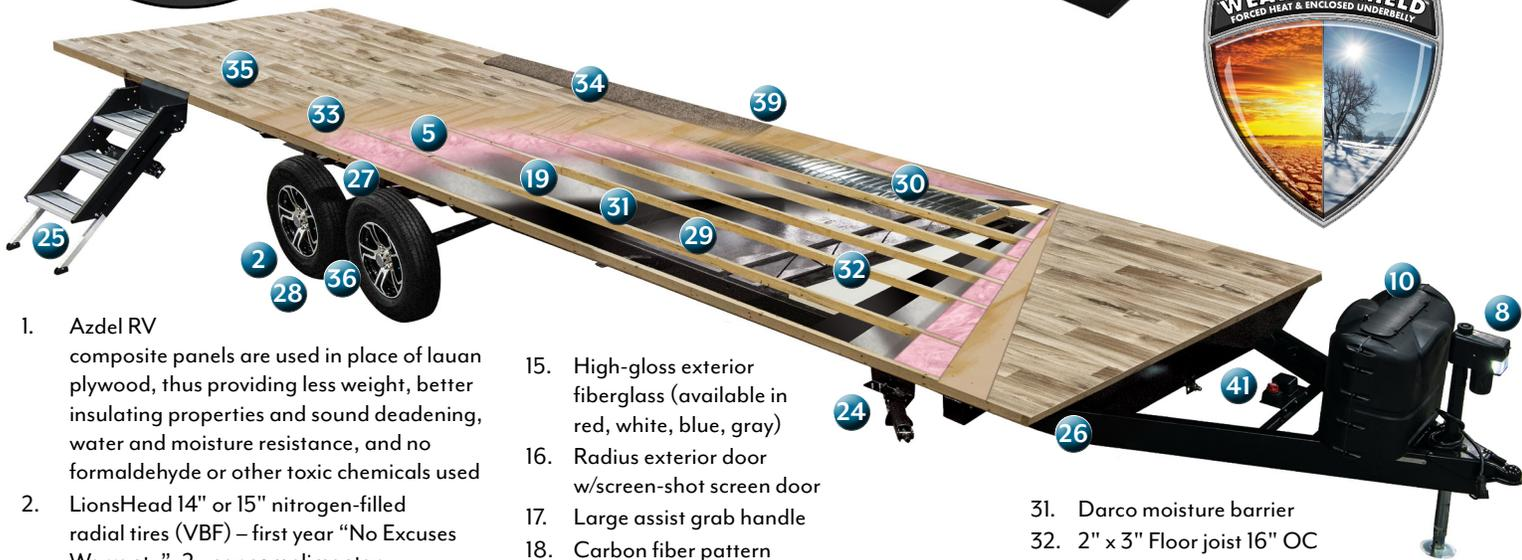
1. Azdel RV composite panels are used in place of luan plywood, thus providing less weight, better insulating properties and sound deadening, water and moisture resistance, and no formaldehyde or other toxic chemicals used
