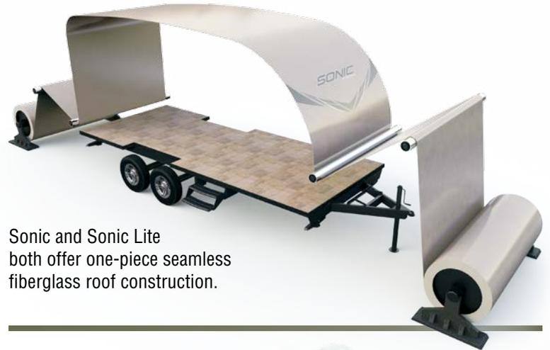
Sonic and Sonic Lite both offer one-piece seamless fiberglass roof construction.
