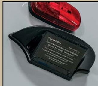
Backup camera prep allows for easy installation of the optional backup camera.
