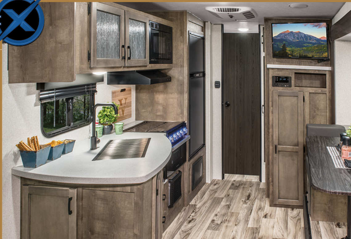
Sonic X interiors include solid wood cabinets with roller ball bearing drawer guides, a large undermount stainless steel single bowl sink, and two interior speakers.
